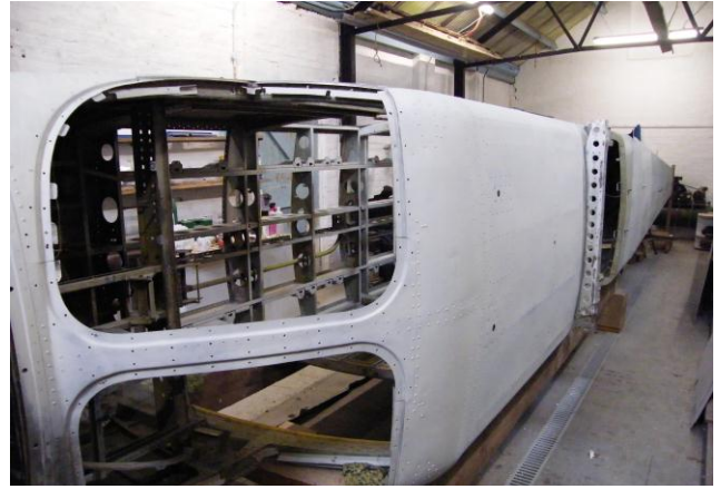
Cabin roof and windscreen surround structure has been de-corroded and primed
