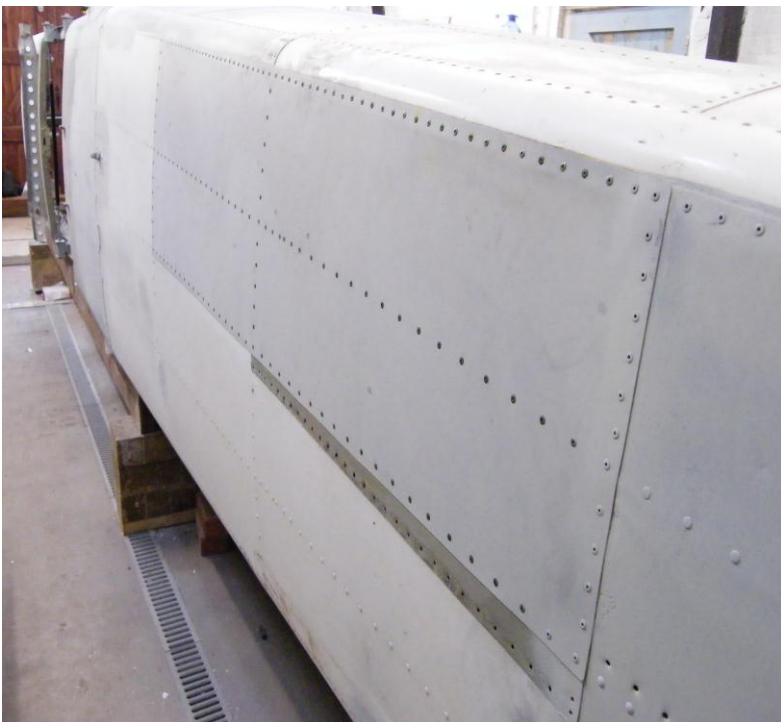
View of the replacement skin on the top of the rear fuselage and a new top corner section to repair the damage when another aircraft was blown into VCN in a storm in Puerto Rico.
