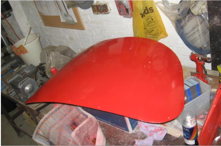
Painting the avionics bay cover to obtain the required high quality finish turned out to be a labour of love for Bob Wilson
