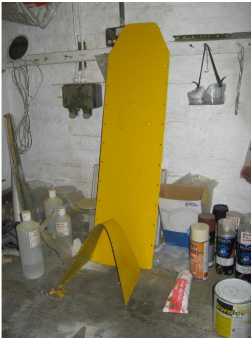
Closure panel and part of the dorsal fairing have been painted and are now ready for installation.
