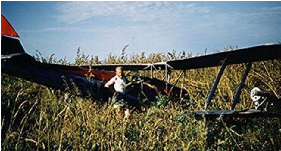
Sorting out Tiger Moth G-AMVF after a forced landing following a bird strike
