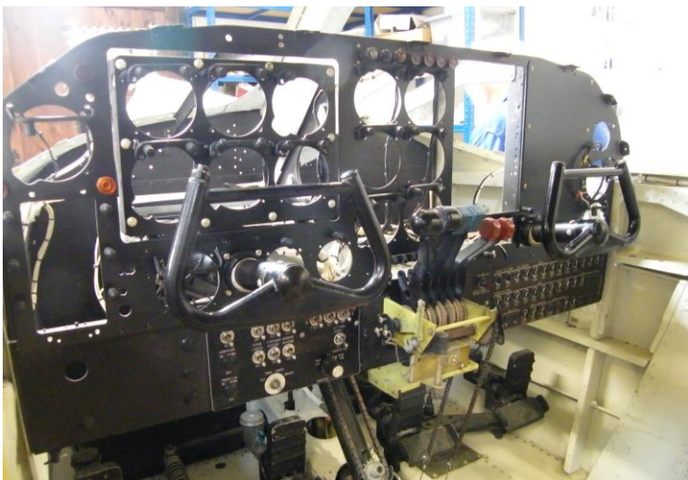
The pilot's and co-pilot's control wheels have now been installed. Bryan Groves has rigged a spring loaded pulley system for the aileron cables so that the control wheels can be operated in a representative way.
