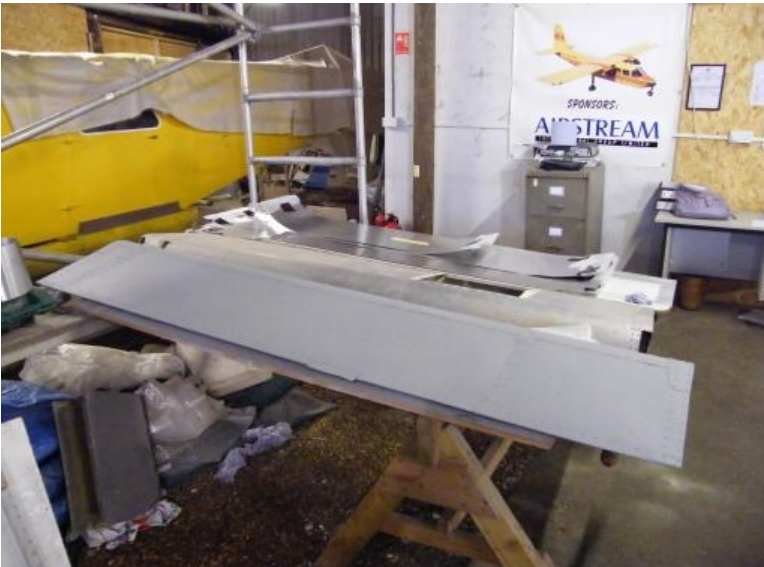
Starboard aileron is now etch primed and ready for spray painting.
