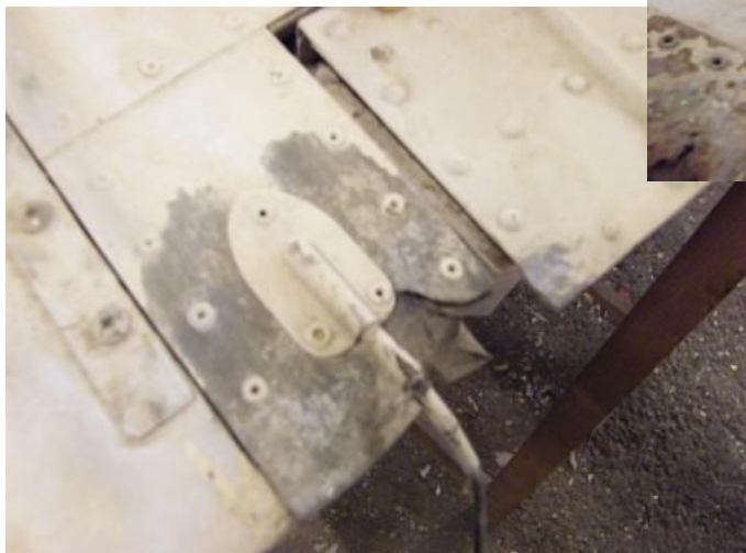
The crushed supporting structure adjacent to the mass balance housing is shown on the right
