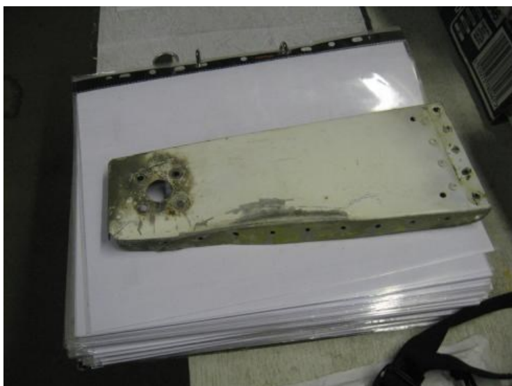
View of the damaged and distorted mass balance arm side panel after removal. It is necessary to ensure the correct alignment of the bushes for the elevator hinge bolts when the side panel has been repaired and re-installed.
