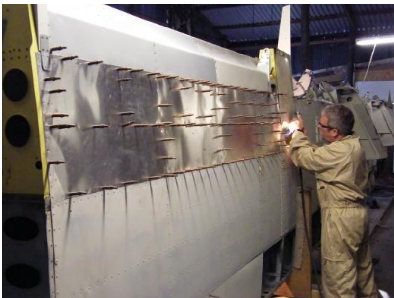
Another view of the wing skin with Mark Porter supporting the new panel while the last of the fixing holes are drilled through—the rippling will be corrected during final installation and riveting.
