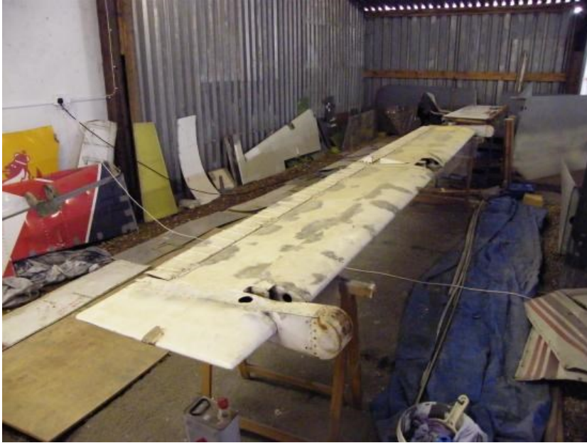
The elevator is now being de-corroded, stripped of old paint together with repairs to the mass balance housing and surrounding structure and a buckled section of the trim tab trailing edge.
