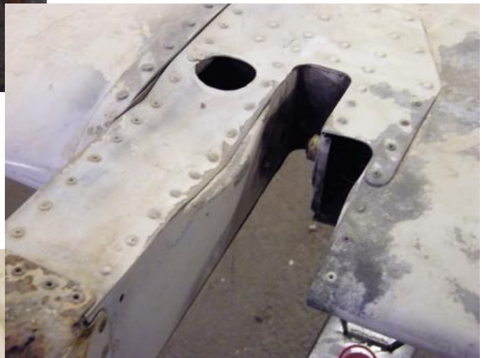
The view on the left shows the damaged trailing edge alongside the static electricity discharge wick. The planned repair action is to make a small replacement skin section.
