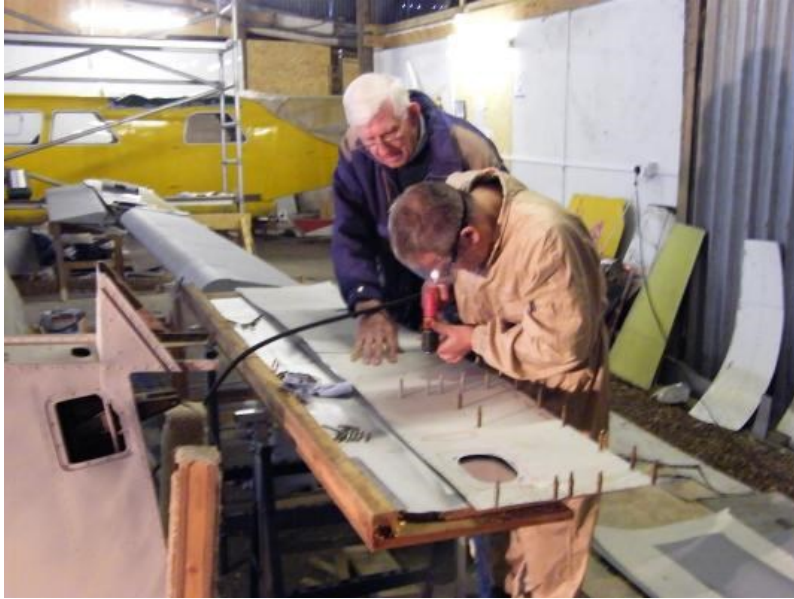
Bob Ward (left) and Mark Porter prepare a new skin for installation using the old skin as a template for drilling the reference fixing holes
