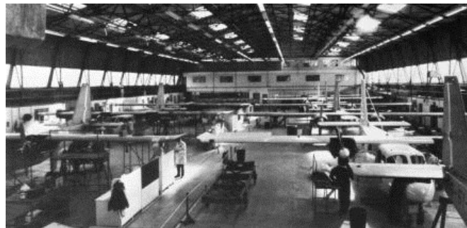
The assembly line at Bembridge where Islanders go through seven stages of assembly prior to weighing and flight test
