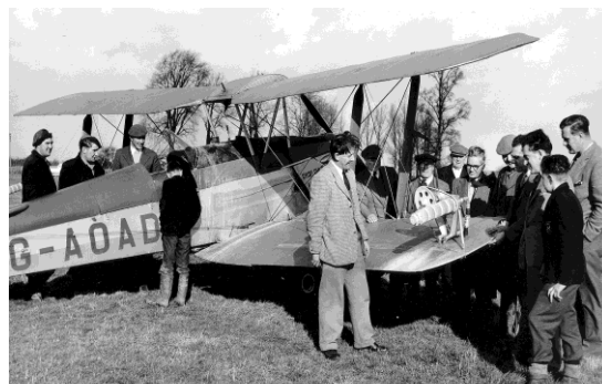
Crop Culture Tiger Moth fitted with Micronair rotary atomisers.
