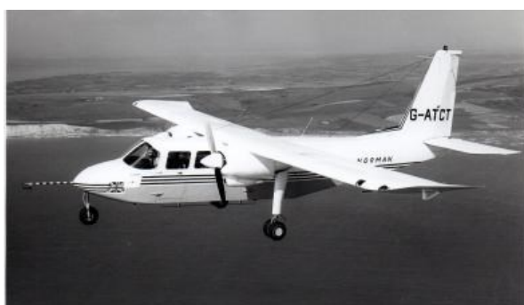
Prototype BN-2 G-ATCT on flight test after modification to install 260 hp Lycoming engines.
