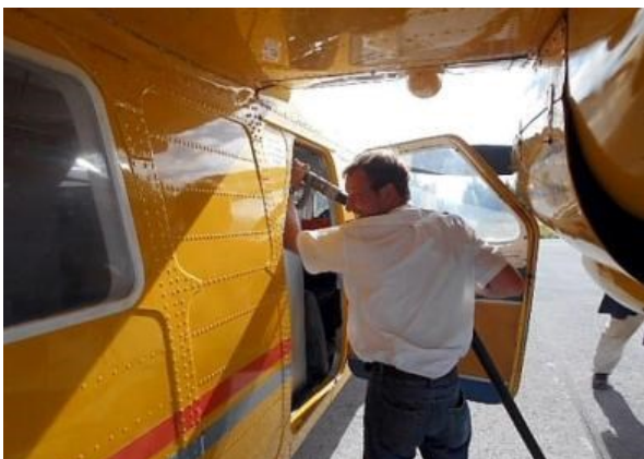
Tony Deamer at Kona refuelling the ferry tanks fitted in the cabin for the delivery flight.
