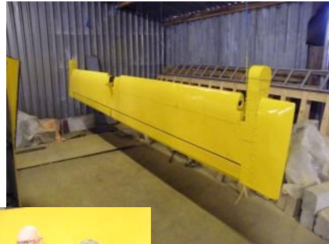
View of the elevator after top coat spray painting.
