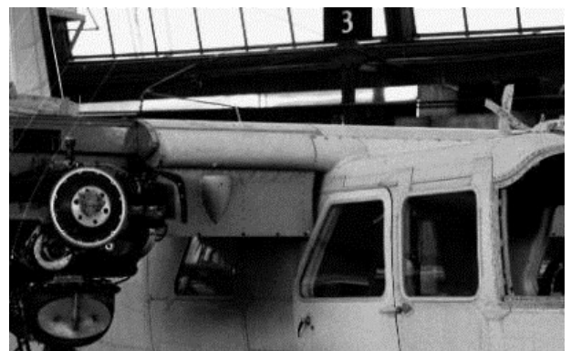
Wing leading edge droop section to reduce the stalling speed was installed inboard of the engine.
