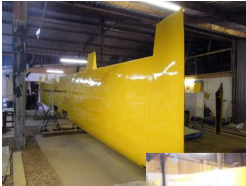
View of the wing upper surface after top coat spray painting.
