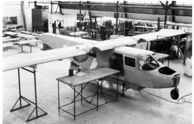
Initially Islander fuselages and wings delivered by BHC to Bembridge to the BHC receiving area before entering the line
