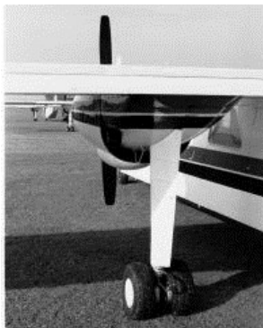
Views right and above show the later production configuration of engine cowlings, rear nacelle fairings and main landing gear leg fairings.
