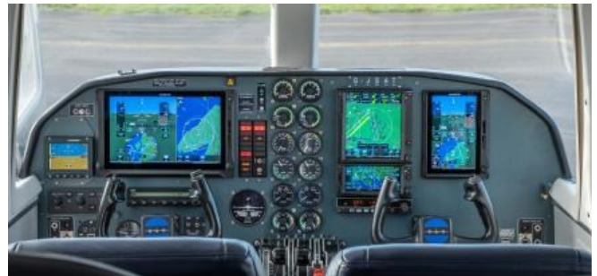
Garmin G600 TXi installation in BN-2T G-JSAT (B-N).
