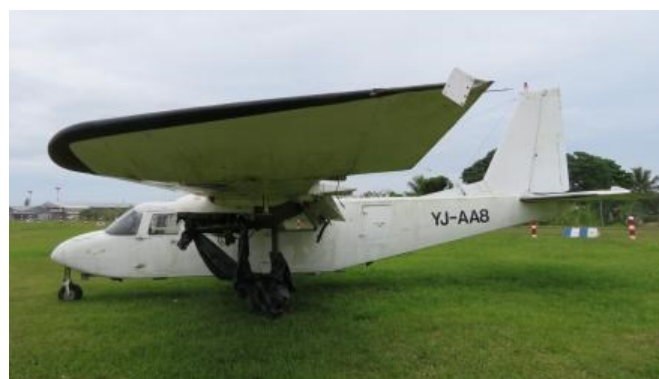
Islander YJ-AA8, of unknown ownership, has no engines and appears to be stripped of useable components. Note the label attached to the outer edge of the port wing. This informs the unknown owner that the port aileron has been removed, presumably for use on another airframe!
