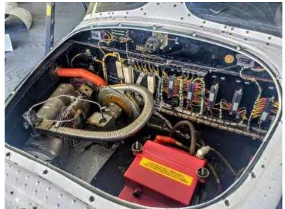
Heating equipment in the nose avionics bay of Islander C-GRNZ was installed by B-N Aircraft Leasing, West Kelowna, BC (Great River Air).
