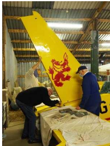
Left: Steve Cooley (l) and Mark Porter are seen here during removal of the rudder (Bryan Groves).
