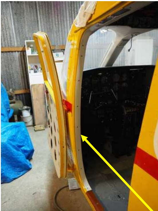
Left: View of the pilot's door with its door aperture surround installed. Right: View of Starboard passenger door with door aperture surround in place Door aperture surrounds were installed by Paul Thomasson and Keith Winter before the Islander was taken apart for the move from Brickfields workshop (Bryan Groves).
