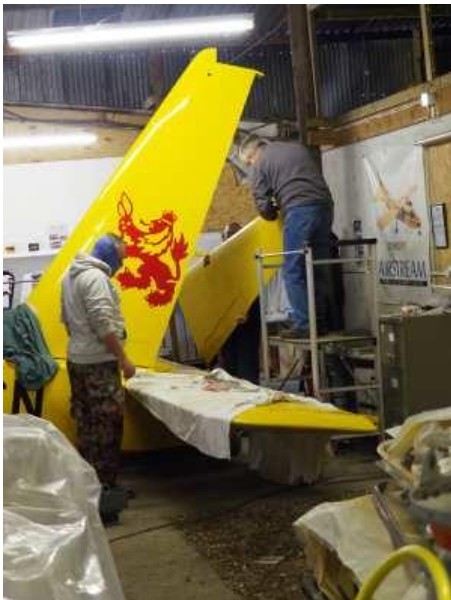
Left: Steve Cooley (l) and Mark Porter are seen here during removal of the rudder (Bryan Groves).
