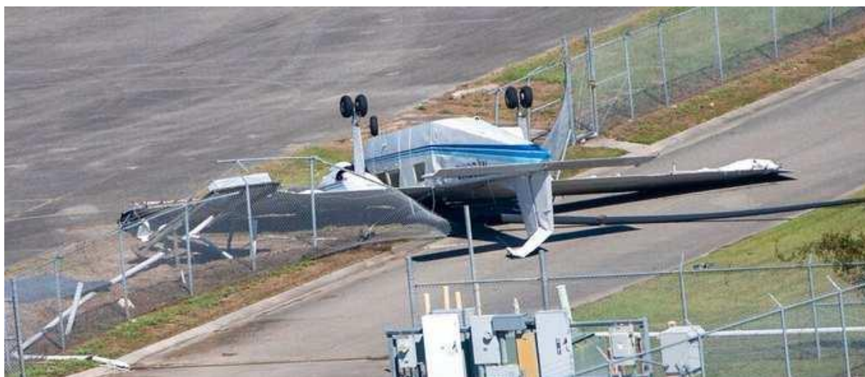
N706MC (c/n 883) awaiting recovery after being damaged during Hurricane Zeta at Lakefront Airport, New Orleans, Louisiana, USA. (BNH Collection)
