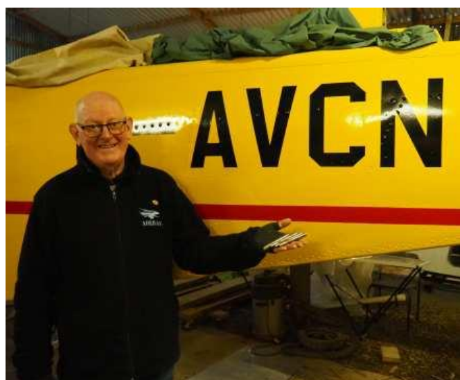
Paul Thomasson with the four taper pins that joined the wing and fuselage. Taper pins had been installed, instead of bolts, in anticipation of the fact that the aircraft would have to be taken apart for transport. (Bryan Groves).
