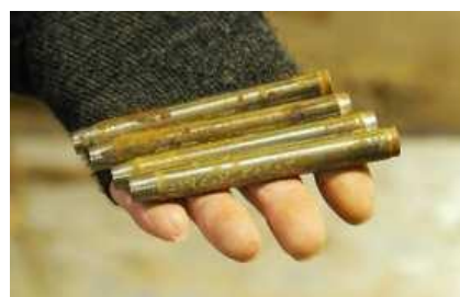
Paul Thomasson with the four taper pins that joined the wing and fuselage. Taper pins had been installed, instead of bolts, in anticipation of the fact that the aircraft would have to be taken apart for transport. (Bryan Groves).
