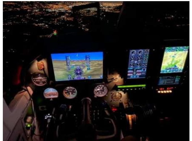
Above: View of the digital instrumentation equipment installed in FIGAS Islander VP-FMC.
