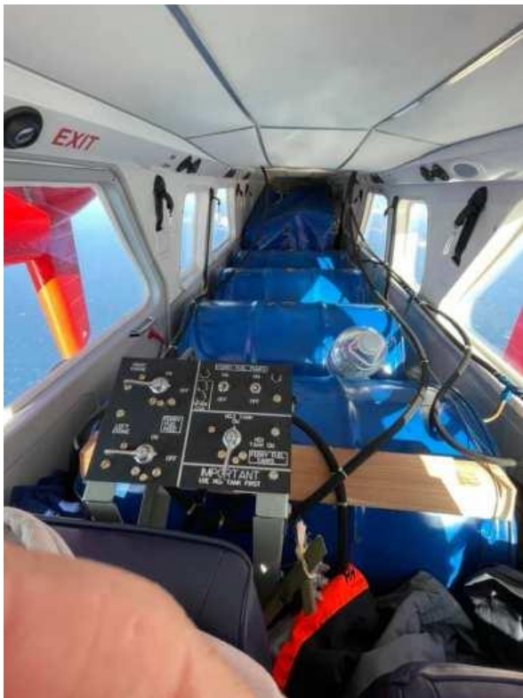
The cabin seating was removed and replaced by the ferry flight fuel system consisting of four fuel tanks and associated valves and fuel supply pipework to give a flying time well in excess of 10 hours for the flight (Mark Eddleston).
