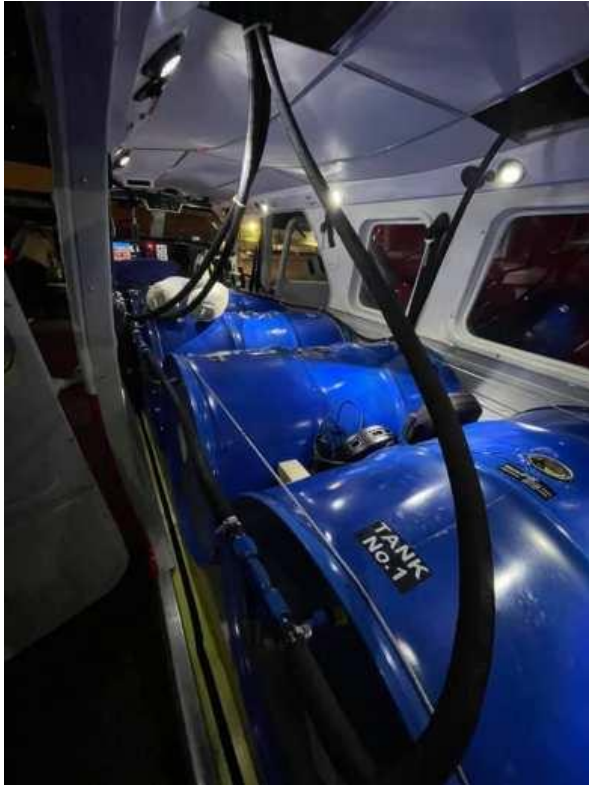
The cabin seating was removed and replaced by the ferry flight fuel system consisting of four fuel tanks and associated valves and fuel supply pipework to give a flying time well in excess of 10 hours for the flight (Mark Eddleston).
