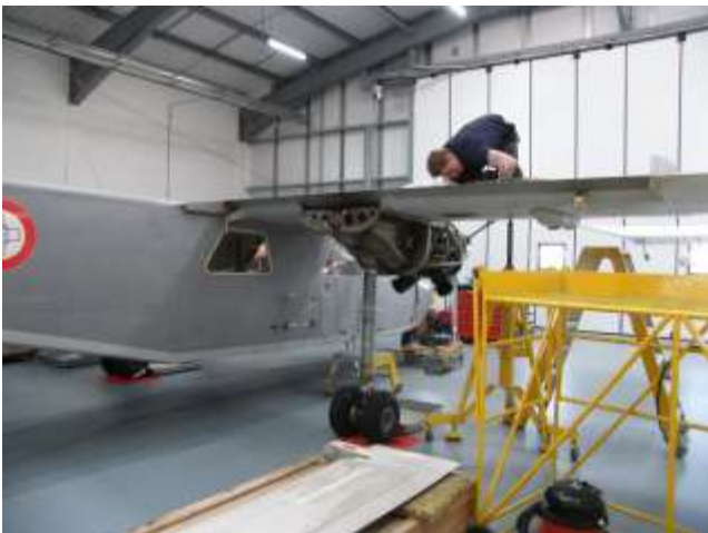
Work in progress in B-N's Hangar 5 on major overhaul and installation of new flight instrumentation and interior trim for Armed Forces Malta BN-2T A9819 (BNAPS).
