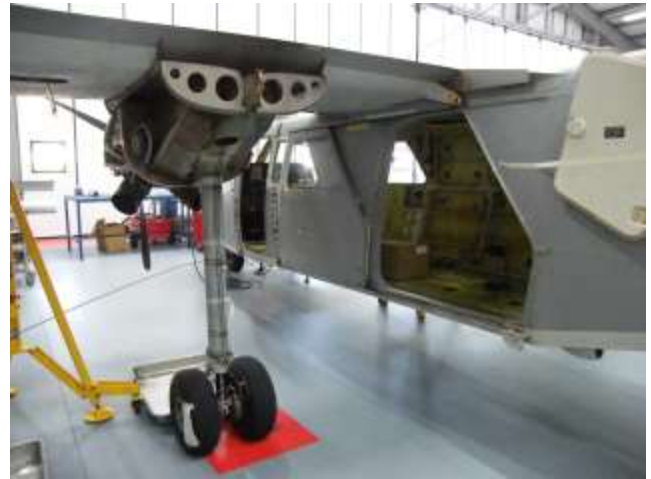
Work in progress in B-N's Hangar 5 on major overhaul and installation of new flight instrumentation and interior trim for Armed Forces Malta BN-2T A9819 (BNAPS).
