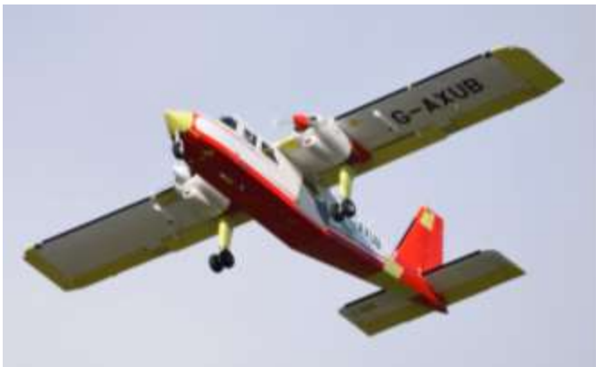
Islander G-AXUB seen taking off on 14 October. It is evident that replacement nose cone, wing tips, main u/c leg fairings, ailerons and flaps were installed during its refurbishment. Also noted was the installation of a standard port rear passenger door (Graham Tiller).
