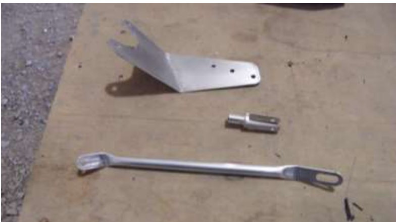
Standard parts proving unavailable, pattern governor control linkage support and fork end fitting have been fabricated by Bryan Groves
