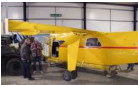
Re-joining the wing and fuselage May
