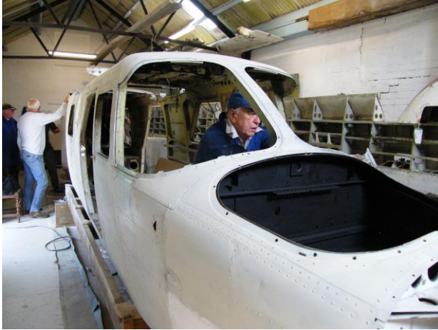
Guy Palmer working on the instrument panel mounting frame and a view of the re-painted avionics bay.
