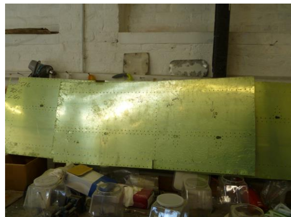
Replacement floor section drilled ready for surface preparation and etch priming
