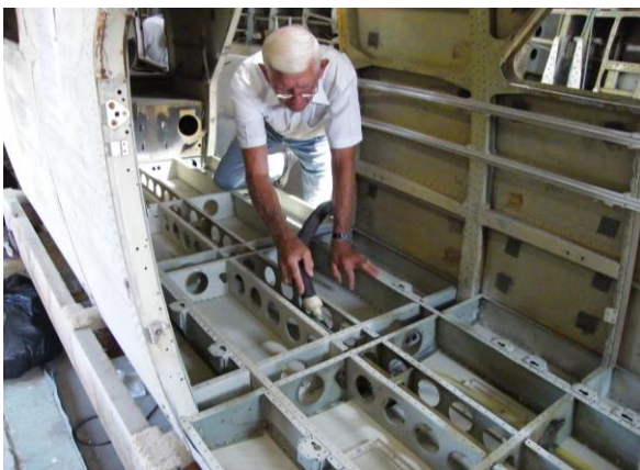
Bob Ward cleaning out the under-floor void prior to fitting replacement floor.
