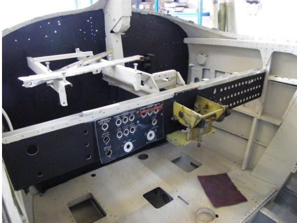
Refurbished instrument panel area and support frames.
