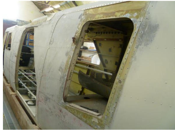
Baggage bay door aperture being de-corroded and repaired.
