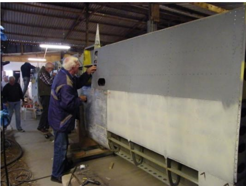
Bob Ward is seen here working on the port outer wing top surface skin re-installation.
