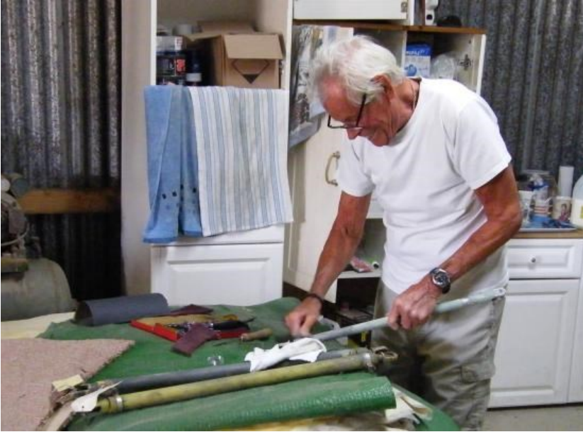
Paul Brook is seen here cleaning and re-furbishing one of the flap control rods
