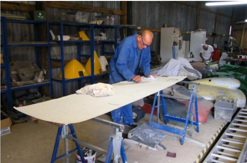
Keith Winter prepares another wing skin ready for installation.
