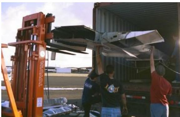
The wing had to be inserted into the container in a horizontal position and turned to the vertical once inside.
