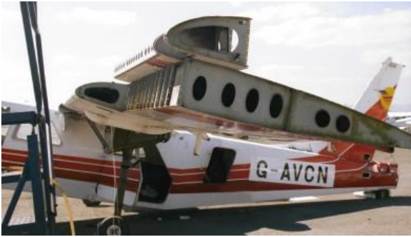
View of the Port wing after removal of a section of the wing box and leading edge.
