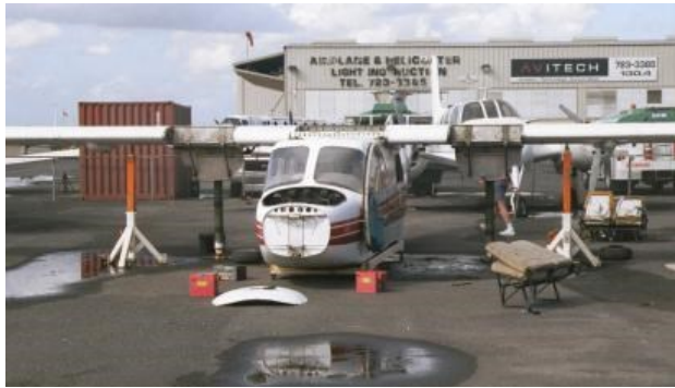
Seats and external parts are removed and wing stands now in place
