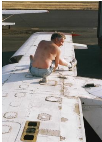
Peter Graham, working on the wing structure around the wing bolts.
