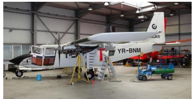
INCAS Islander YR-BNM during its 2 yearly corrosion check.
