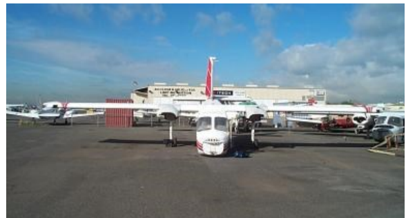
Head on view of Islander c/n 3 at Isla Grande Airport Puerto Rico. Engines, nose landing gear and instruments were all missing
