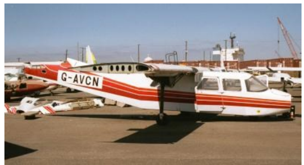
Islander c/n 3 with the fin removed prior to starting the process of separating the wing and fuselage.
