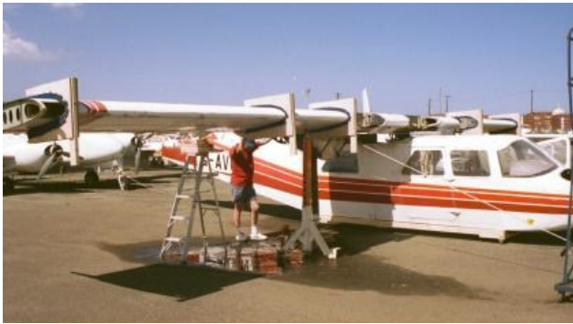
Vertical wing support cradles were fabricated and are seen here being fitted in place.
