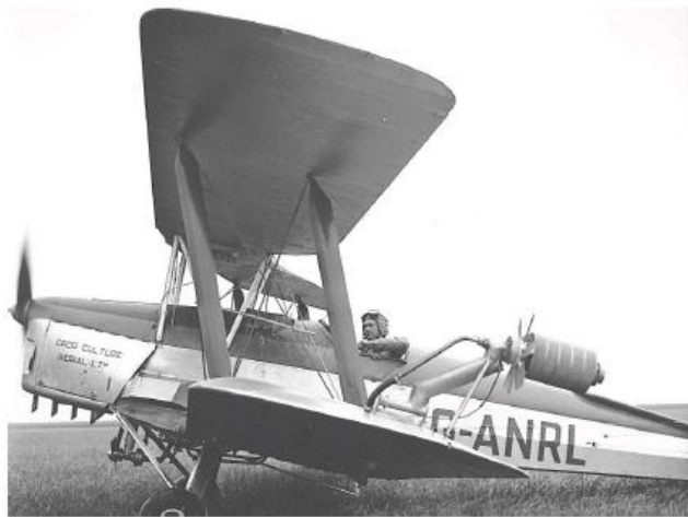
Jim McMahon in Tiger Moth G-ANRL with Micronair spray units fitted P Gatrell
