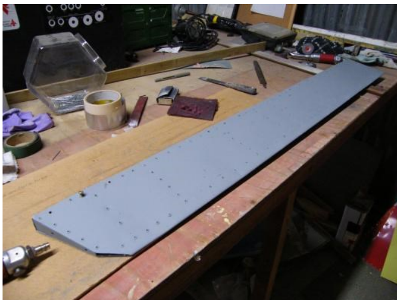
Keith Winter has completed fabrication of a replacement rudder trim tab. The tab has also been etch primed ready for spray painting.
