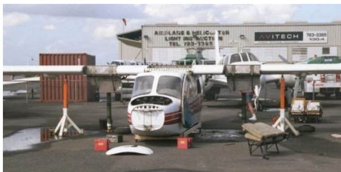
N290VL/G-AVCN is seen here being dismantled and then stowed in a freight container for shipment to the UK (BN Historians)
