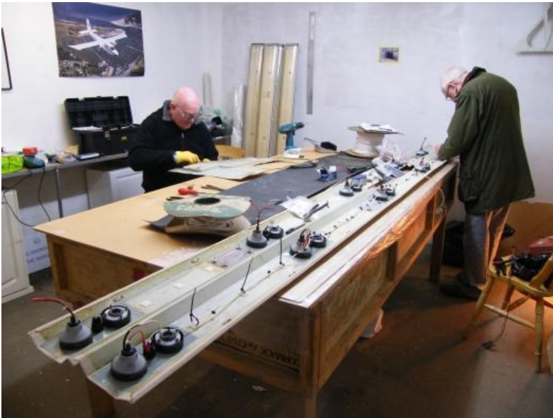
View of work under way in the trim shop. Bryan Groves (right) wired up the switches and lights on the passenger service unit trim panels. Paul Thomasson is working on one of the passenger door trim cards.
