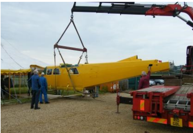
The restored fuselage is seen here being offloaded to go on show at "Islander 50" (BNAPS Archive)
