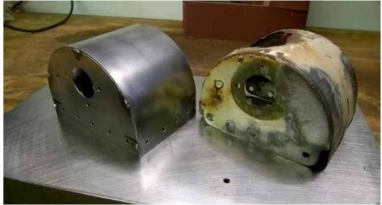
View above shows the new steel mass balance cap made by Ralph alongside the existing badly corroded item.
