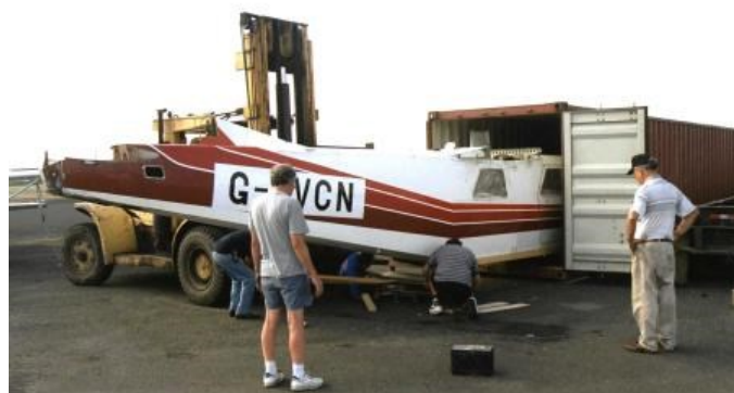
N290VL/G-AVCN is seen here being dismantled and then stowed in a freight container for shipment to the UK (BN Historians)
