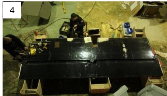
4 - Tail plane (from Spectre Islander) and elevator assembled.
