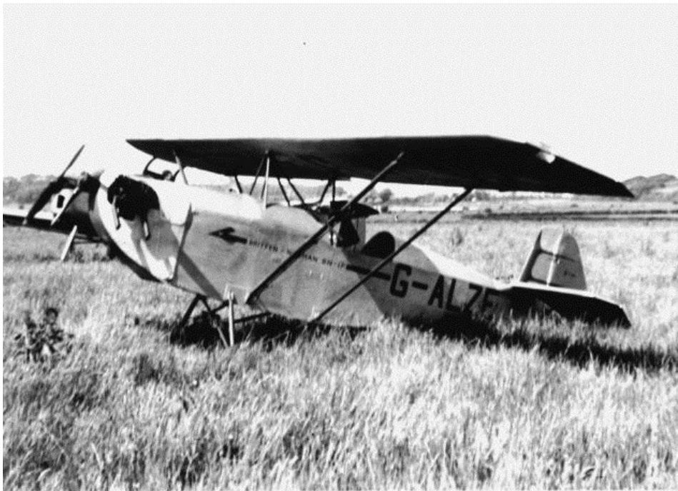
The BN-1F "Finibee", G-ALZE, is seen here at Bembridge Airport in early May 1951. It has been fitted with a 65hp Lycoming engine together with an enlarged rudder as a result of earlier test "hops" in August 1950 (Peter Gatrell).
