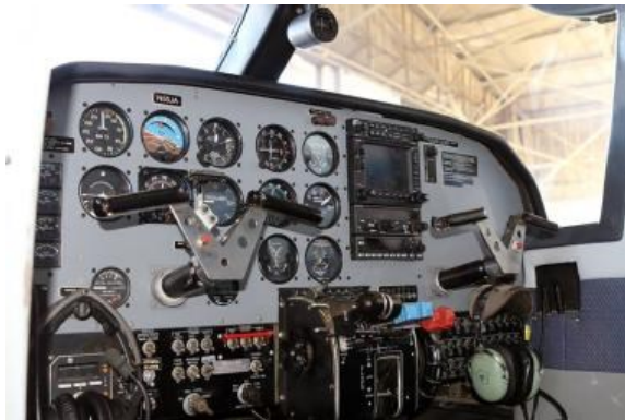
View of the cockpit of Islander N55JA showing original instruments and "rams horn" controls.
