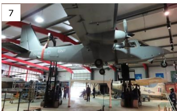
7 - Lift carried out using two fork lift trucks.
