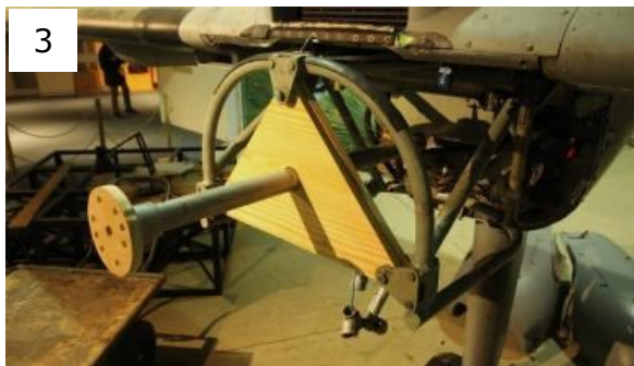
3 - Propeller mounting structure installation.
