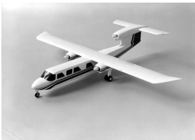
Britten-Norman company model of the BN-2A Mk.III Islander concept - note the limited fin area that was later increased as a result of flight testing (Taffy Lloyd family)
