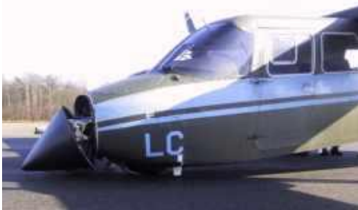
Views of the fuselage damage and the nose landing gear caused by the hard landing.
