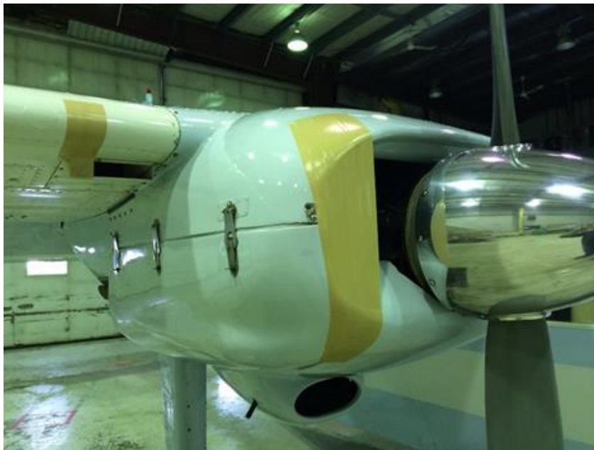
During the stopover at Sept-Iles duct tape was used to reduce the size of the cooling air inlets in the engine cowlings.
