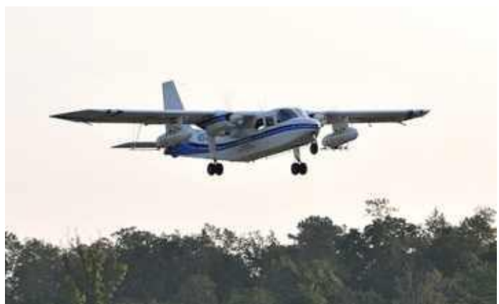
Islander N50693 with spray booms installed in place of Micronair rotary atomisers (Ed Foster).
