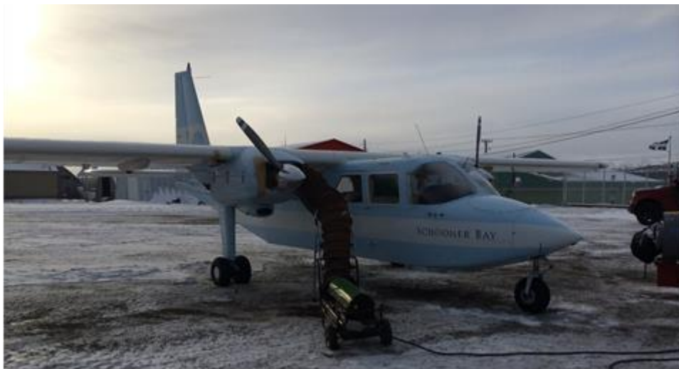
Hot air blower in use to warm up engines of the aircraft after a cold night outside in snowy conditions at Sept-Iles
