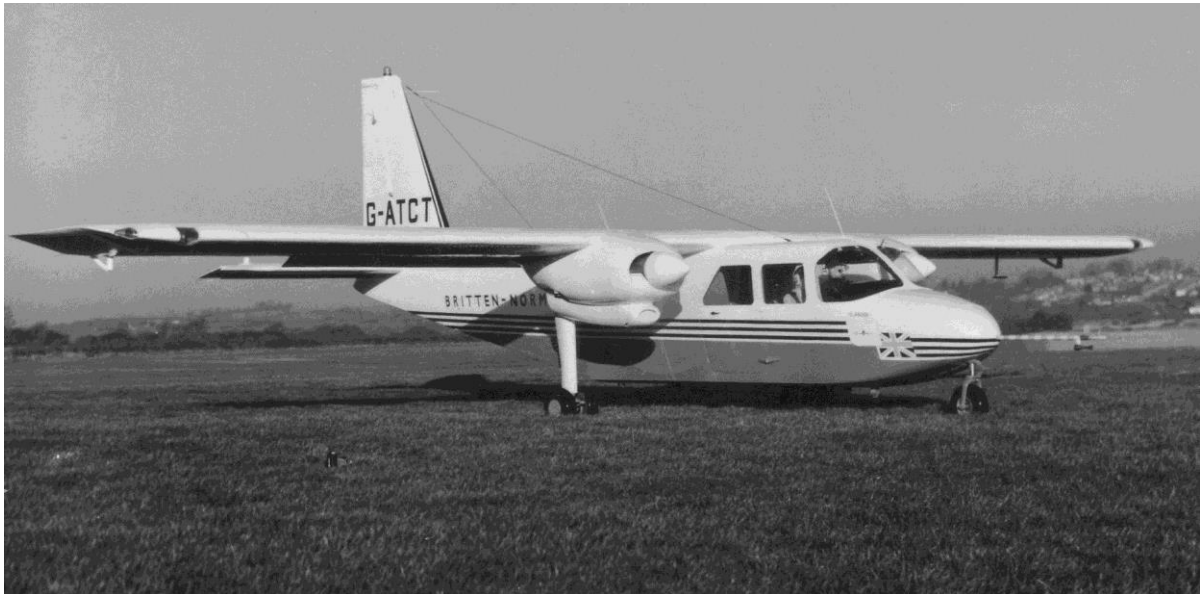
BN-2 Islander G-ATCT now fitted with the Lycoming O-540 engines ready to continue the flight test programme in early 1966 (BW Collection)
