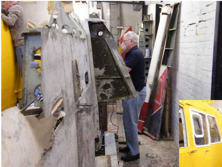
Jeni Gallagher is seen here tackling the messy process of applying paint stripper to remove old paint from the wing's upper surface.
