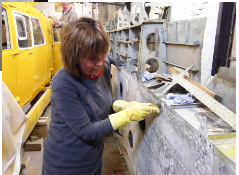
Jeni Gallagher is seen here tackling the messy process of applying paint stripper to remove old paint from the wing's upper surface.
