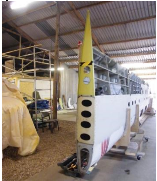
Maurice Dyer has recently joined the restoration team and is seen here working on the wing to remove damaged formers (left) Replacement formers were then installed (right)
