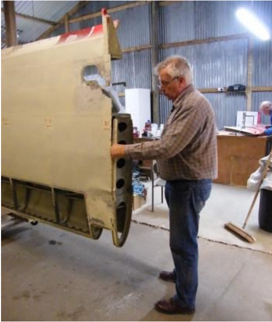
Maurice Dyer has recently joined the restoration team and is seen here working on the wing to remove damaged formers (left) Replacement formers were then installed (right)
