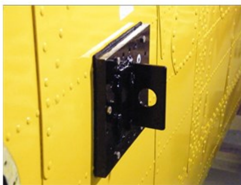
Left - This shows one of two lifting plates fitted in place of access panels on the wing's upper surface adjacent to strong points around the main landing gear tube support structure. The existing access panel cover plates were used as templates for drilling the lifting plate fixing bolt holes.
