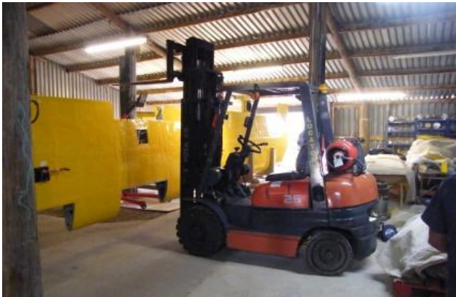
Right: Lift is complete with the wing supported on the adjustable wing trestles, now mounted on wheeled bases.
