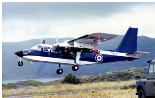
BN-2T Islander ZF573 in its earlier role as an MoD Trials Aircraft for the air launched Stingray torpedo (B-N).
