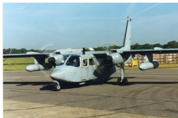
AAC Islander AL.1 with under-wing fuel tanks installed (BNAPS Archive Collection)
