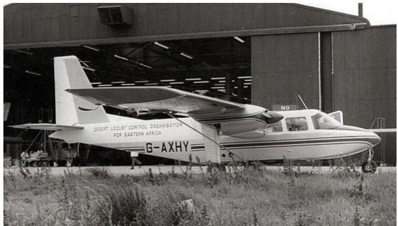
Islander G-AXHY, c/n 601, is seen here at Bembridge having the Micronair spray equipment installed (BNAPS Archive Collection).
