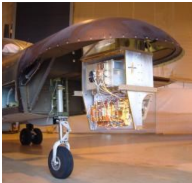
ZG889 with EADS Astrium synthetic aperture radar installed (BNAPS Archive Collection)
