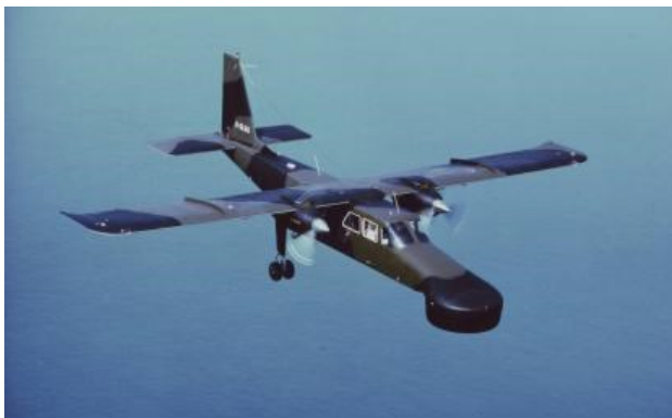
MoD BN-2T Islander G-DLRA/ZG989 with the CASTOR "platypus" radar nose shape (BNAPS Archive Collection)
