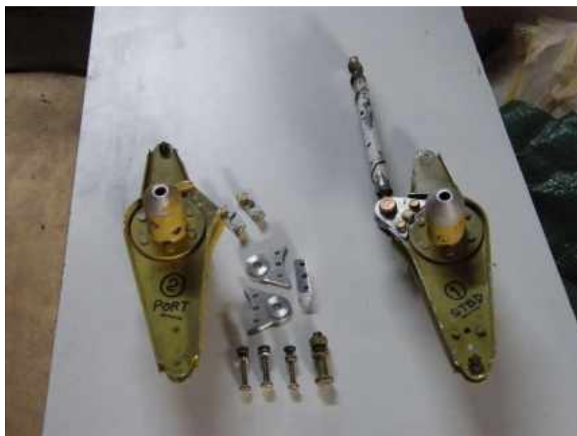
Repaired Aileron Lever Assemblies
