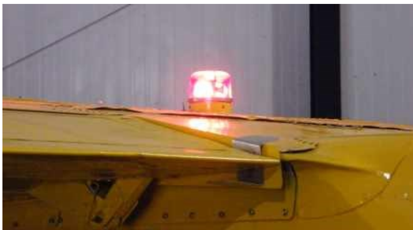
Anti-Collision Beacon unit under test
