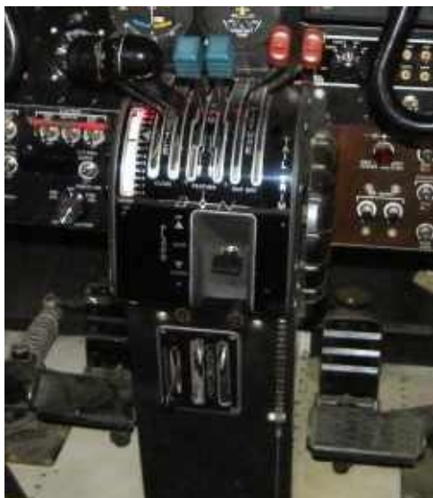
Left – Refurbished engine control pedestal Right- Fuel Cocks.
