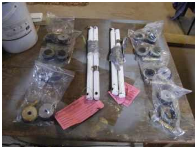
Refurbished Struts and Mounting Lugs and replacement rubber mounts ready for installation
