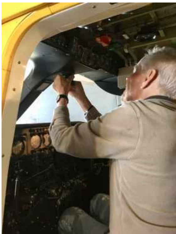
Left - Paul Brook installed the E2B Standby Compass after installing the trim capping section around the central wind screen pillar (Bob Wilson)
