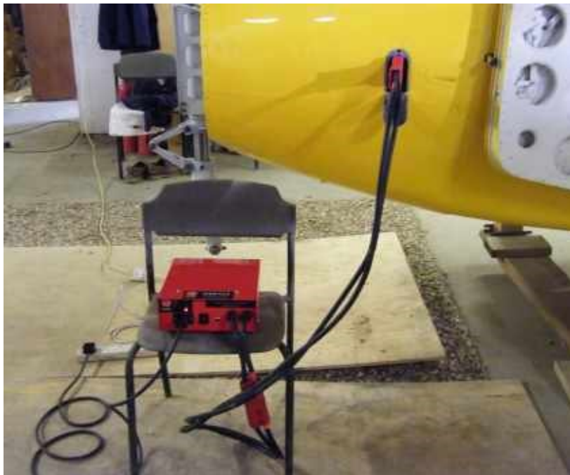
External 24 Volt DC Power Supply.
