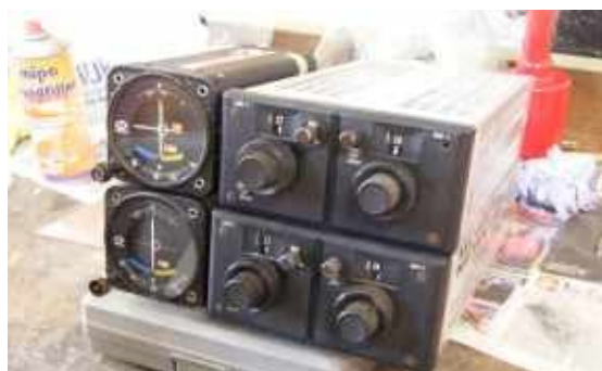
Narco K12A Communication/Navigation equipment as installed.
