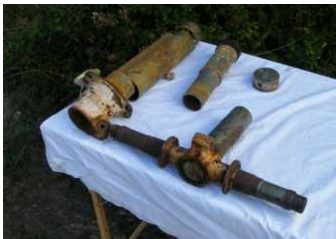
Existing landing gear components were too badly corroded for re-use.
