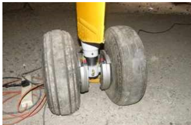
View of main landing gear with brake discs and calipers installed
