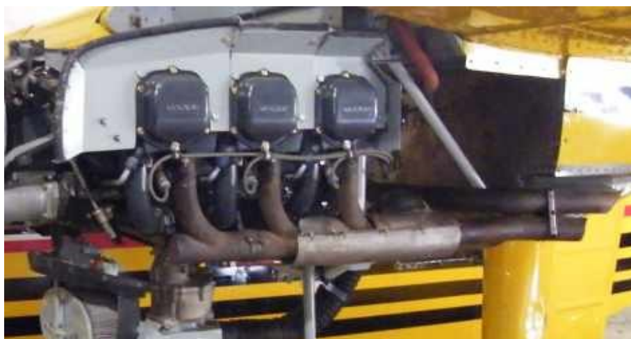
View of Port Engine Exhaust System installation
