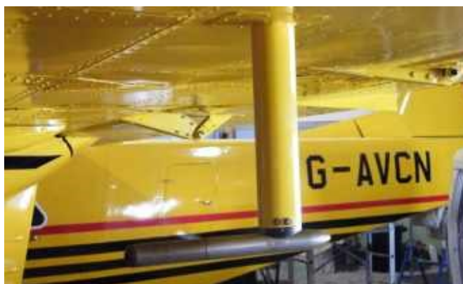
Pitot Static Head as installed after repair and refurbishments
