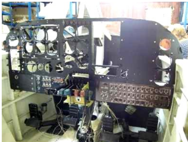
Main instrument panel and controls at an early stage of rebuild and refurbishment.
