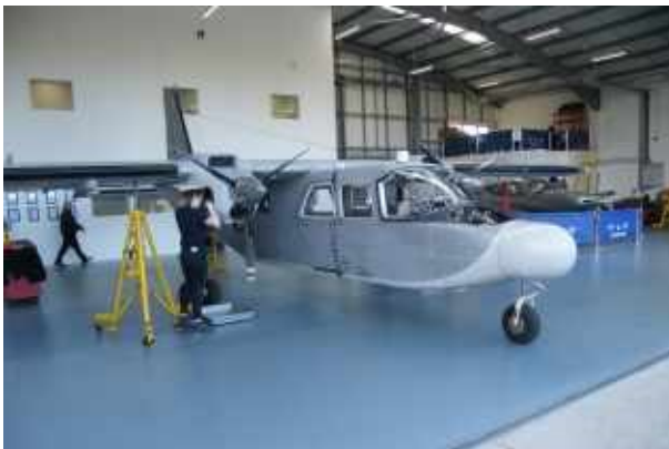
In Hangar 5 the Armed Forces of Malta BN-2T AS9819, c/n 2156, was seen being made ready to go to Biggin Hill for re-painting after completion of a major overhaul, upgrade of avionics and instrumentation and a new interior (BNAPS).
