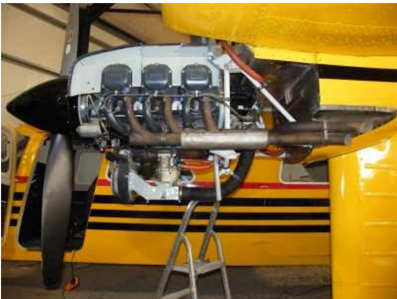
Side view of the port engine as engine dressing work nears completion.
