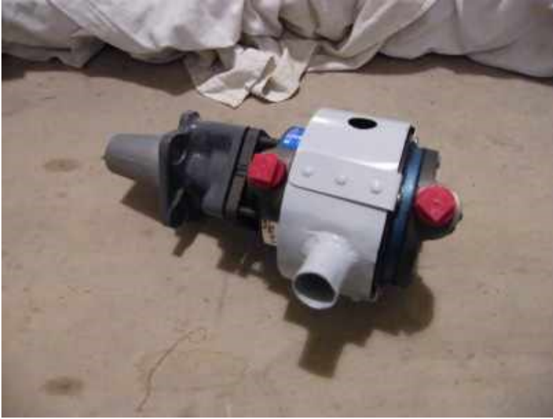
Vacuum Pump fitted with the recently acquired adaptor and heatshield ready for installation
