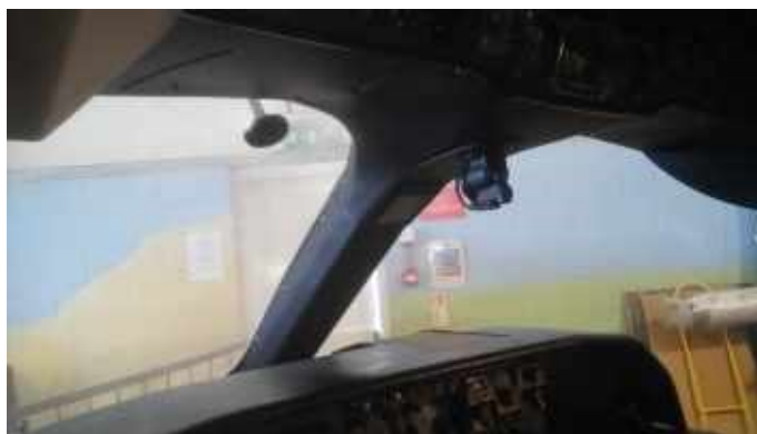
Above – View of the pillar trim and E2B Standby Compass after installation (Guy Palmer).
