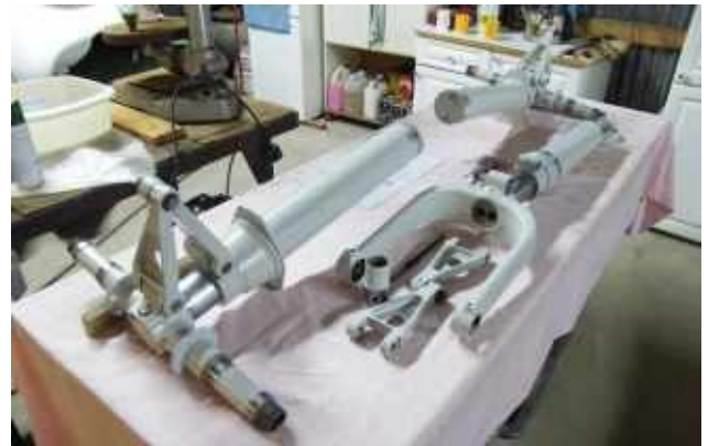
Rebuilt landing gear components ready for installation
