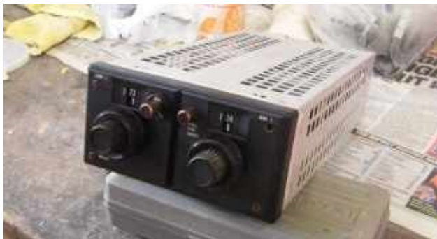
Narco K12A Communication/Navigation equipment as installed.
