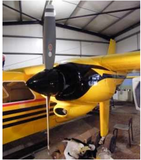
View of Port Engine with Propeller, Spinner and engine cowlings installed
