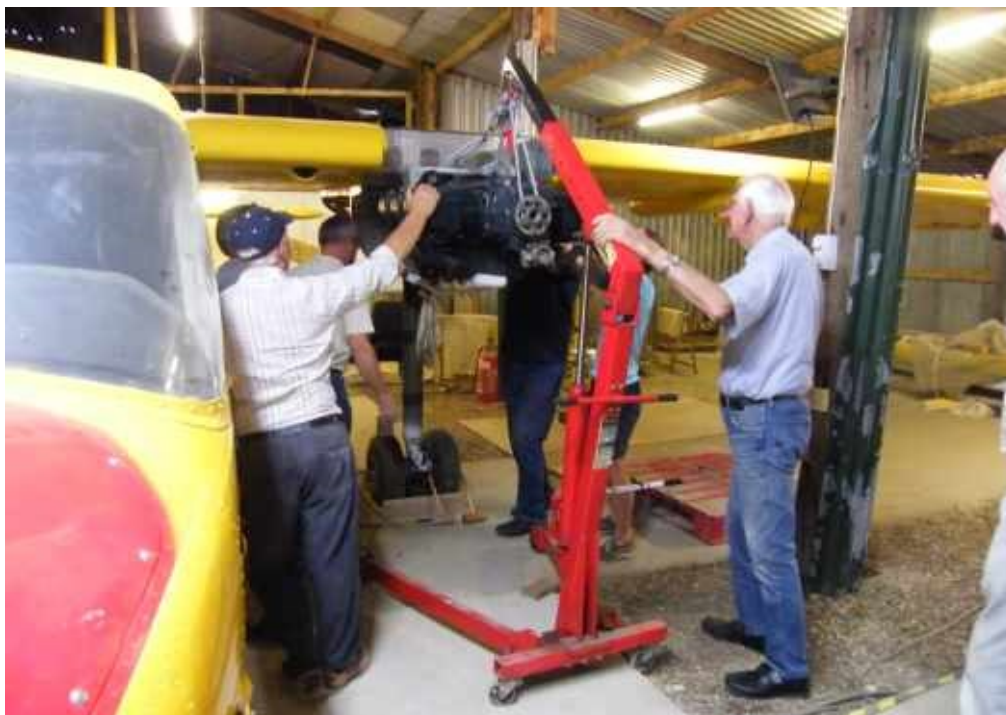
Initial trial installation of Port Engine in progress.
