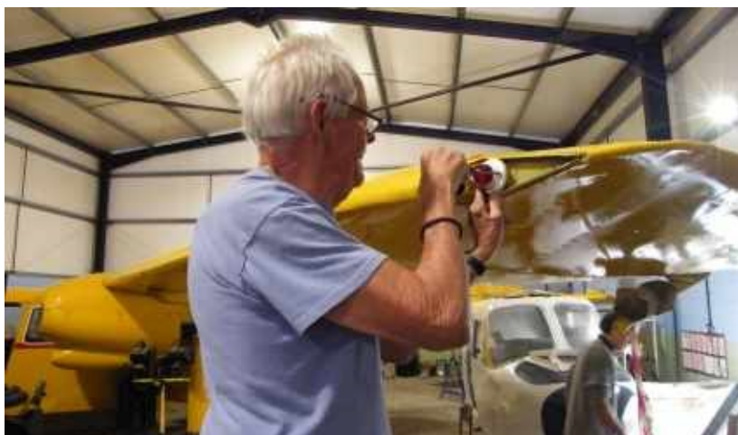
Port navigation light unit being installed
