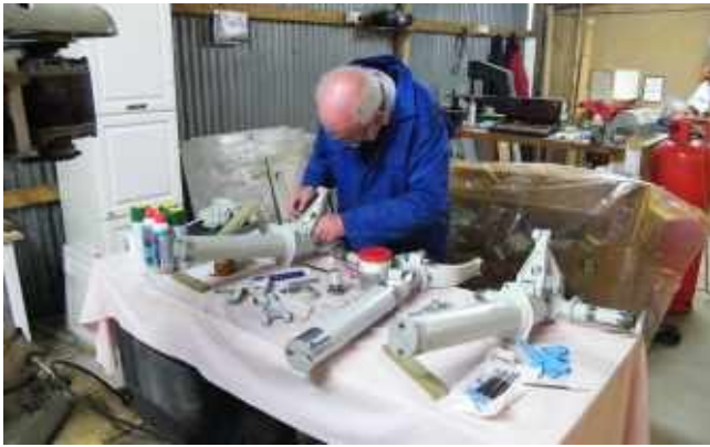
Bryan Groves installed replacements seals and re-assembled landing gear components
