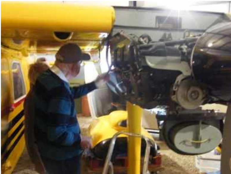
Bryan Groves continued with installation of fuel, air and inlet hoses and ancillary items as part of the port engine dressing work
