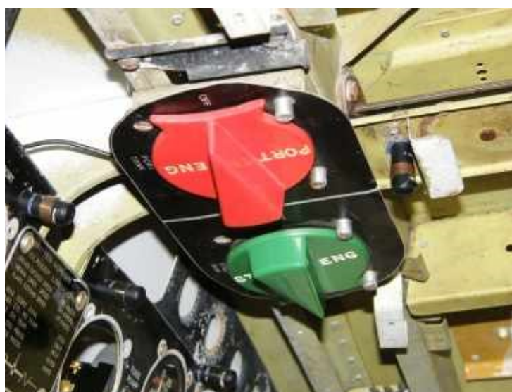
Left – Refurbished engine control pedestal Right- Fuel Cocks.
