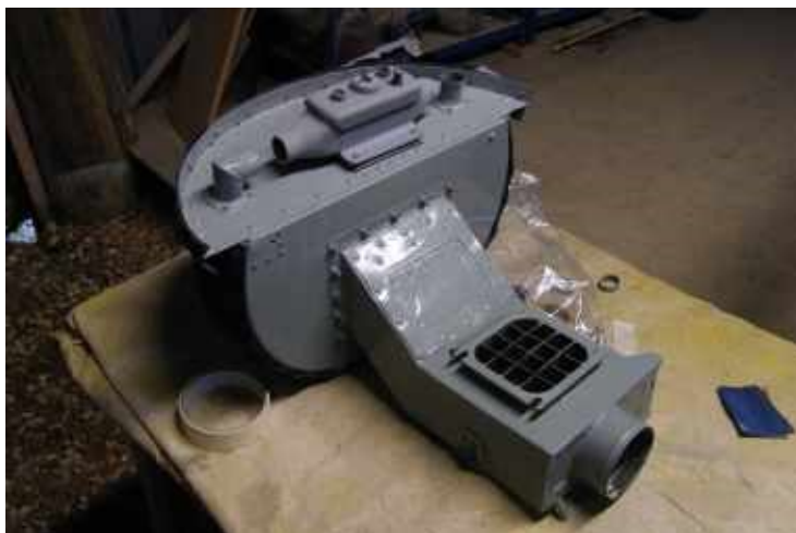
Refurbished Air Box Assembly
