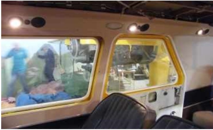
Passenger Service Unit lighting under test
