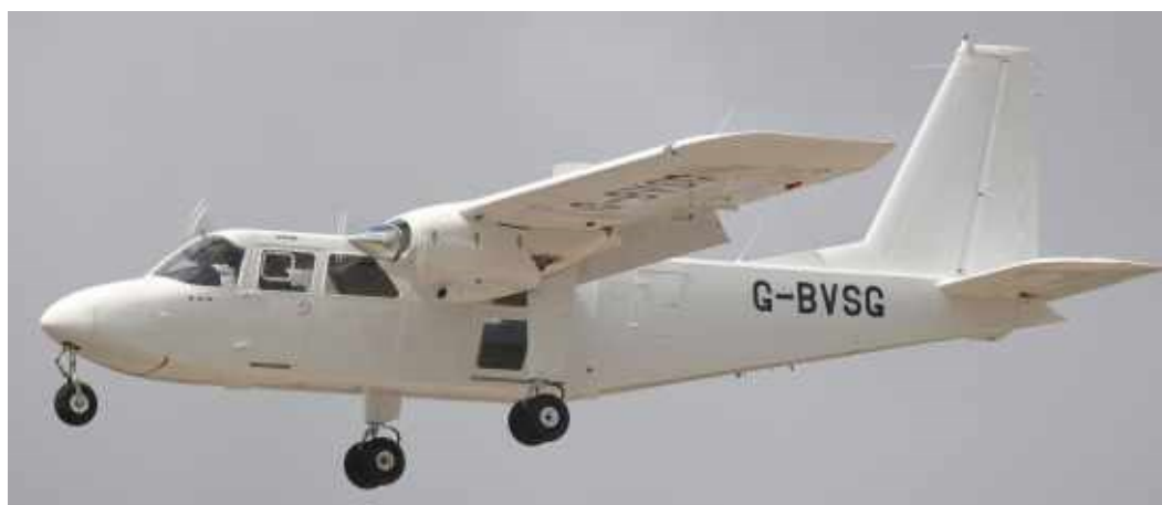
G-BVSG during its first flight since rebuild at Solent. Note the wing fence. (Rich Davies)
