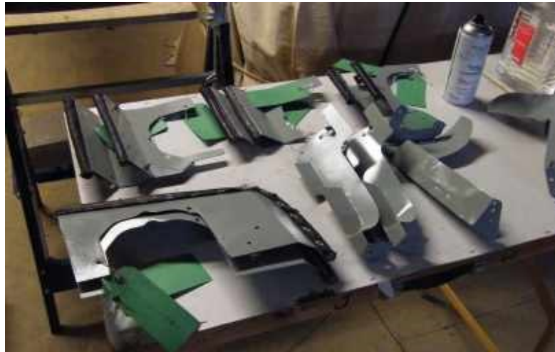
Refurbished Engine Baffles ready for installation
