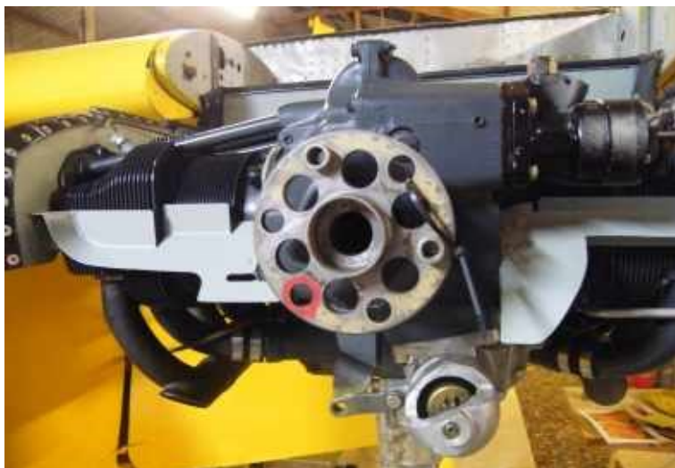
View of the Propeller Mounting Flange and Bushes that required re-positioning.
