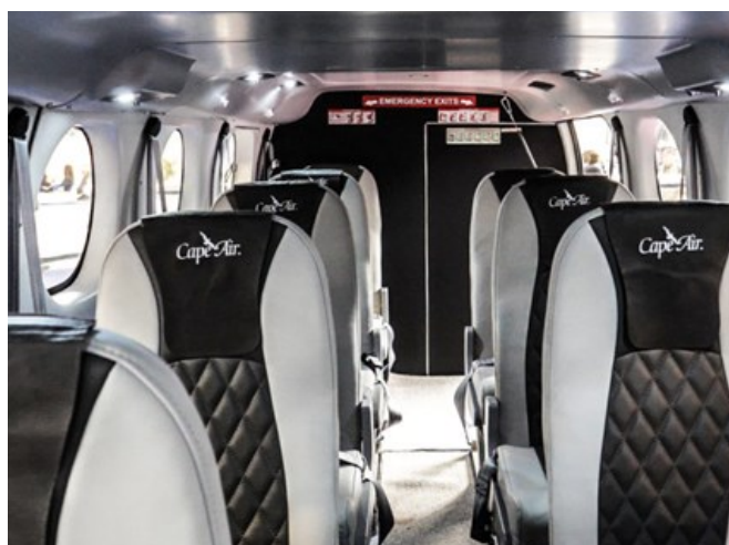
The Traveller's cabin features 11 leather seats with under-seat storage, LED lighting and USB power ports (Tecnam).
