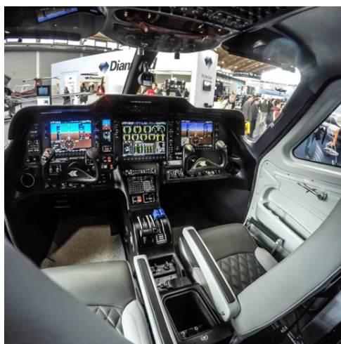
View of the Traveller's flight instrument panel with its Garmin G1000NXi avionics equipment fit installed (Tecnam)
