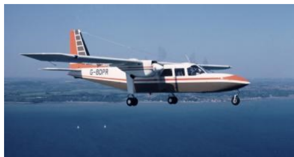
BN-2A-41 Turbo Islander prototype G-BDPR, cn 504, fitted with Lycoming LTP101 turbines, was trialed in April 1977. On test it proved to be overpowered and was withdrawn from use in August 1979 (Ivan Berryman)
