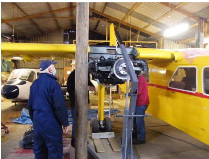
The starboard engine was removed without any significant difficulty.
