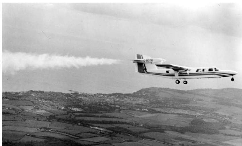
Trislander G-BDTR is seen here on test flight September/ October 1976 over the Isle of Wight with the rocket motor in operation. This could have been a test to ensure the system was fully functional before a demonstration at Farnborough on 18 October 1976 (B-N).
