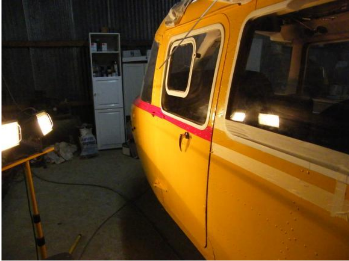
The positioning of the cheat line on the port side of the fuselage was measured and masked off ready for painting using spray cans.
