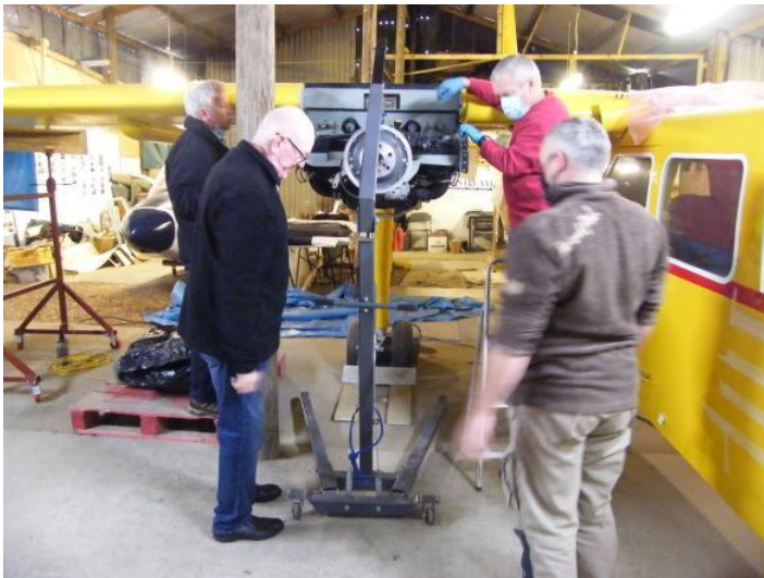
Paul Thomasson, Steve Cooley and Mark Porter are seen here setting up the engine hoist ready for removal of the starboard engine.
