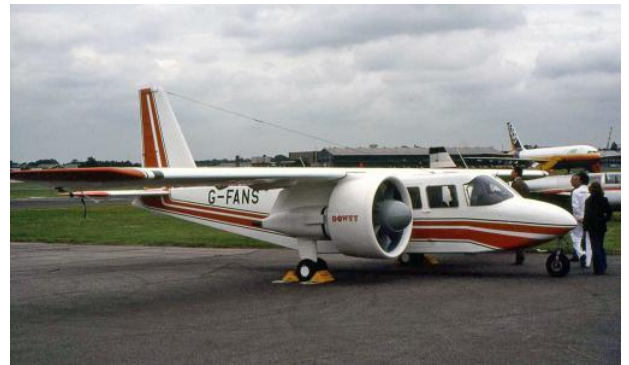
Islander G-FANS with Dowty Rotol Ducted Fan Propulsors installed.
