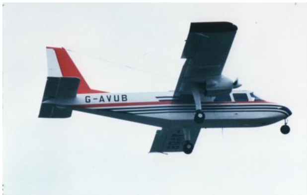
Islander G-AVUB with Continental Turbocharged engines installed.
