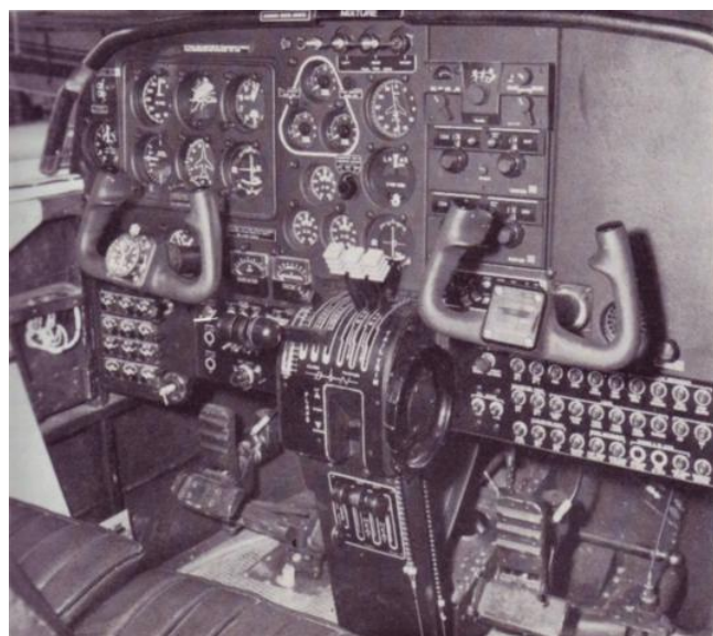
View of instrument panel and controls. Note mixture controls now positioned at the top of the instrument panel and adoption of moulded style control wheels.
