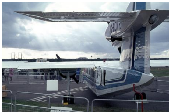
View of the tail section of Trislander G-BDTR showing the rocket motor installation in tail engine pod/tail fairing (BNAPS Archive).
