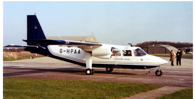
HPASU Islander G-HPAA at Lee in 1993 in its original configuration as a BN-2B-26 with 260hp engines. It was later converted to a BN-2B-20 to take 300 hp engines (Pete Stanton).
