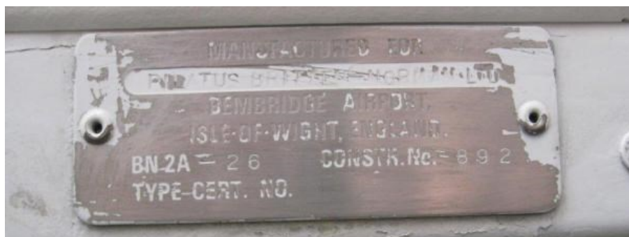
Constructor's plate on XA-PIQ confirms its identity as c/n 892.
