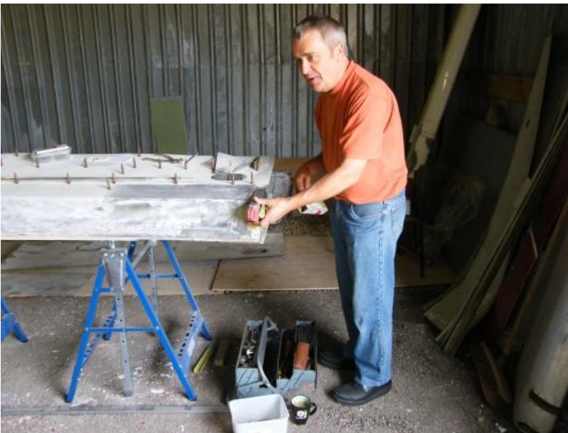
Mark Porter made replacement sheet metal parts for the aileron outboard hinge bearing support and is seen here lining it up with existing fixing holes in the outboard wing rear bay structure.
