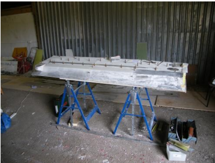
Work on other parts of the wing include (left) installation of new ribs and stringers by Maurice Dyer while Patrick Gallagher continued to re-align and straighten stringers (right) ready for re-fitting restored skins at a later stage.
