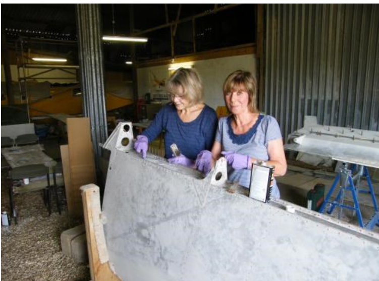
Rita Edgcumbe and Jeni Gallagher removed the last traces of corrosion from the rear closing member of the fin. Etch primer was then applied to make it ready for spray painting
