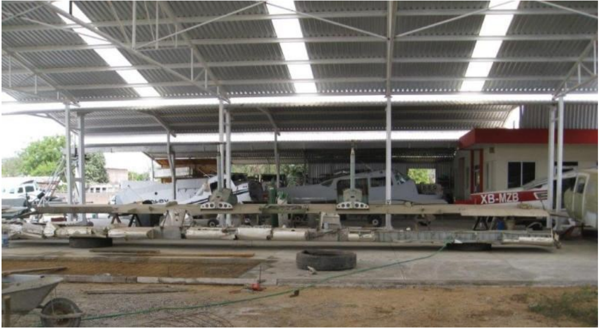
Wing of c/n 24 is stored in the same building as the fuselage. This item looks to be in good condition and has the main undercarriage legs in place.
