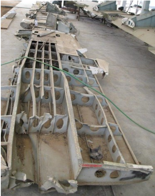
The wing from XA-DEW was severely damaged and appeared to be beyond economic repair
