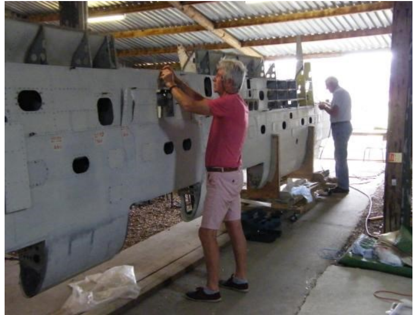
Work on other parts of the wing include (left) installation of new ribs and stringers by Maurice Dyer while Patrick Gallagher continued to re-align and straighten stringers (right) ready for re-fitting restored skins at a later stage.
