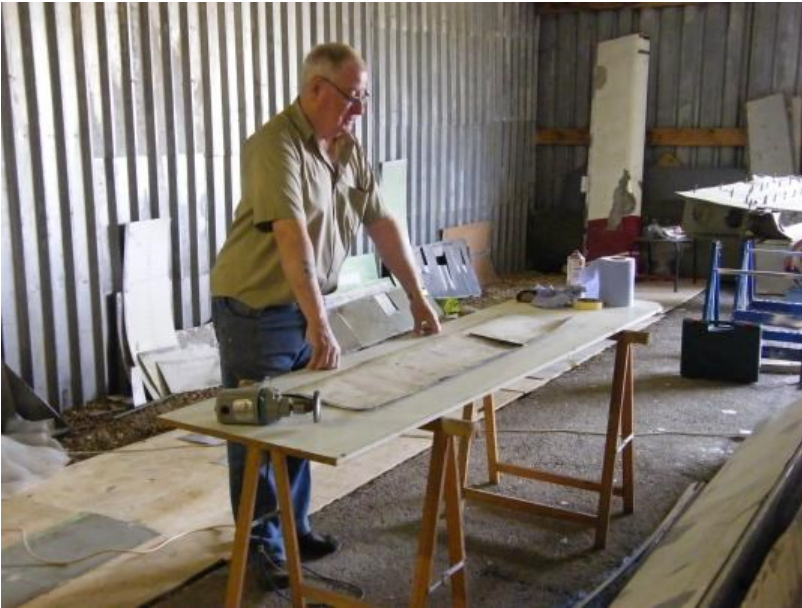
Charles Shiveral worked on one of the smaller wing skins that can be recovered for re-use.
