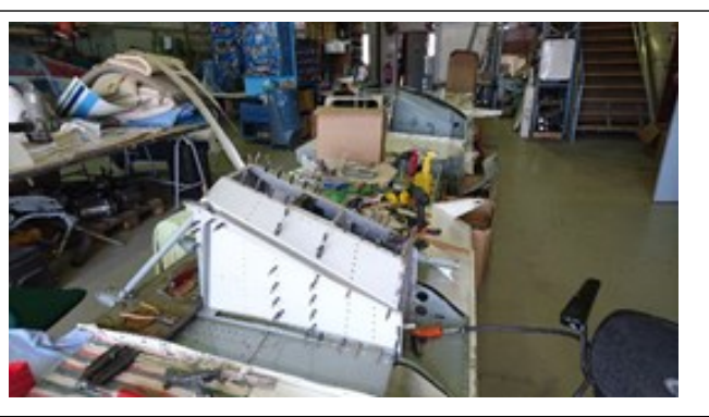
The nearly there and completed nacelle. The quality of the work is testament to the skill and patience of the workforce who have been recruited from the Bodø Luftfartshistoriske Forening.
