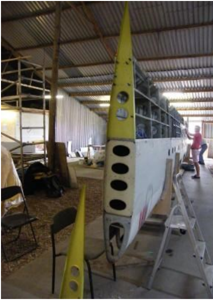
Work on other parts of the wing include (left) installation of new ribs and stringers by Maurice Dyer while Patrick Gallagher continued to re-align and straighten stringers (right) ready for re-fitting restored skins at a later stage.
