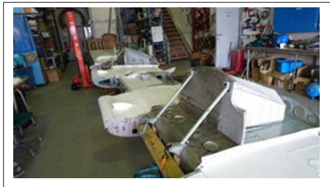
The nearly there and completed nacelle. The quality of the work is testament to the skill and patience of the workforce who have been recruited from the Bodø Luftfartshistoriske Forening.
