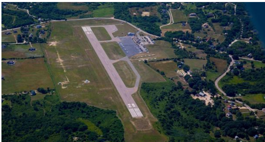
Aerial view of Block Island State Airport's 2,502 by 100 feet (763 x 30 m) runway (Wikipedia).
