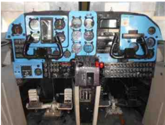
Islander c/n 316 refurbished instrument panel and control position.
