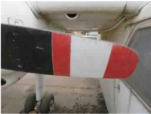
View of the eroded edge of the starboard propeller of Islander XU-MLC/ML501.
