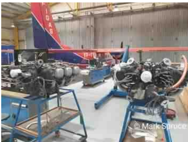
Above: Engines after being removed from VP-FBD. Right: View of Islander VP-FBD during engine change/overhaul work.
