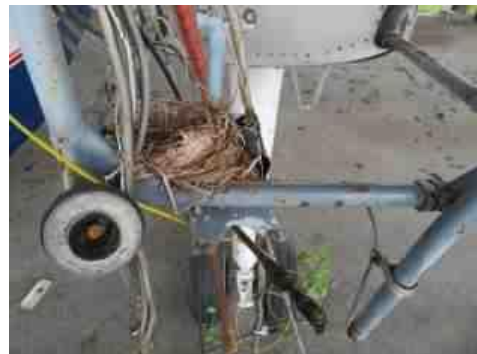
Bird's nest in the port engine mounting of Islander 9M-JPC.
