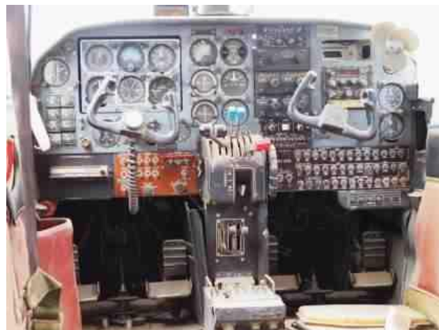
Internal view of Islander XU-MLC/ML501. Switches for the guns have been added on a small floor mounted console.
