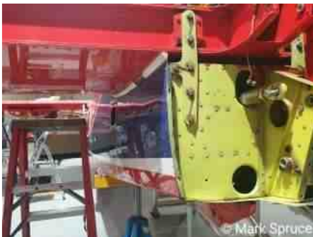
Elevator control rod and surrounding structure access with tail cone removed.
