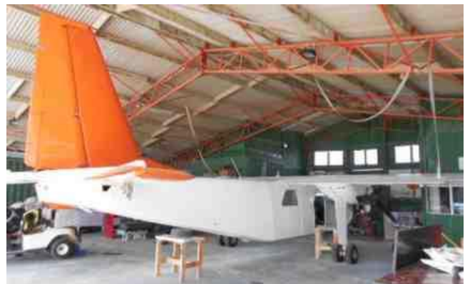
Islander c/n 316 nearing completion of its overhaul.
