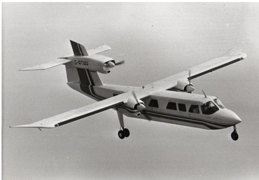
Islander Mk.III G-ATWU in flight. In this view the third engine and angled wing tips can be seen together with its Islander origins (B-N).
