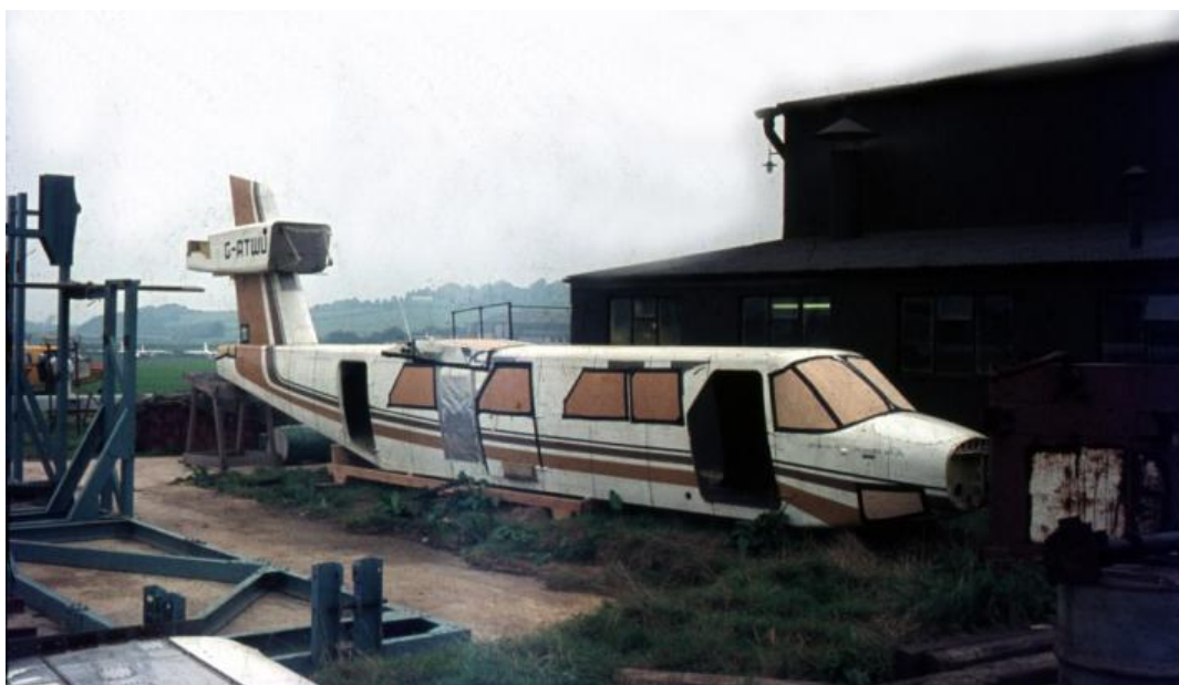
The fuselage of Islander Mk.III G-ATWU when it was used as a structural test specimen at Bembridge in late 1970 (BNAPS Archive Collection).
