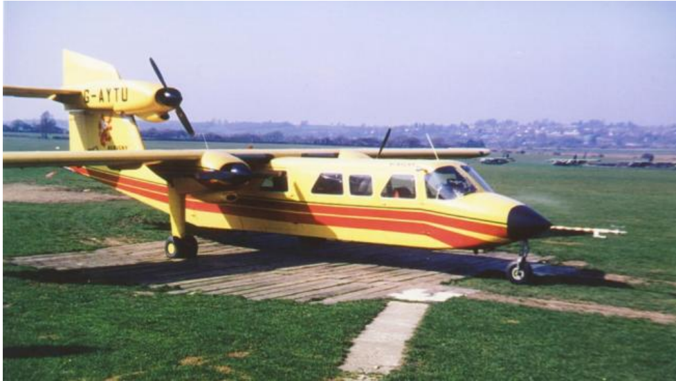
Trislander G-AYTU at Bembridge in early 1971 now painted in Aurigny Air Services colours and fitted with nose mounted test instrumentation probe (BNAPS Archive Collection)
