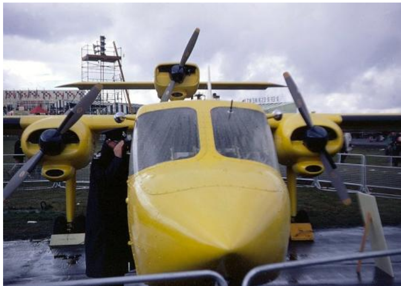
Nose on view of Islander MK.III G-ATWU clearly shows its novel engine configuration (BNAPS Archive Collection).
