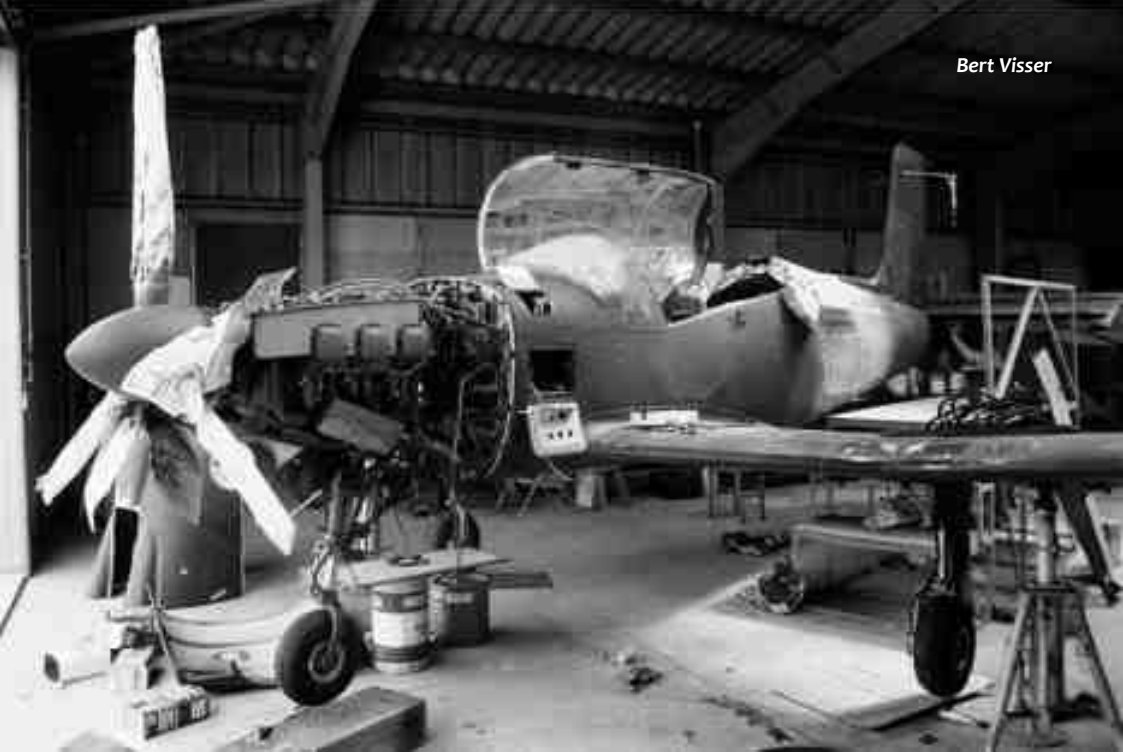
(above) Another view of work in progress on Firecracker G-NDNI. (below) Airframe c/n 003 in process of being built as the first NDN-1T Turbo Firecracker. It is believed that c/n 003 was originally laid down as the second NDN-1 Firecracker. It's likely the c/n 003 identity was superseded and not allocated, as the prototype NDN-1T, registration G-SFTR, is c/n 005 according to the CAA G-INFO database, and c/n 004 seems to have been allocated to Fieldmaster G-NRDC.
