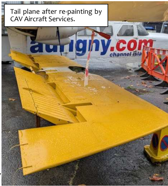
View of tail plane showing patches of primer after treatment of surface corrosion under existing paint.
